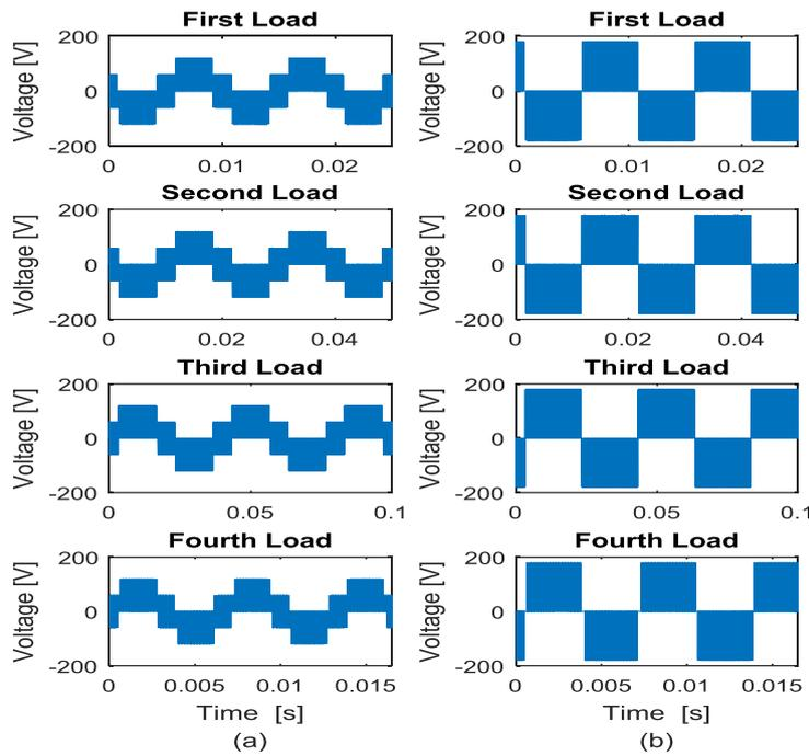
Figure 6. Voltage waveforms for operation mode ‘1111’, (a) phase voltages, (b) line voltages
