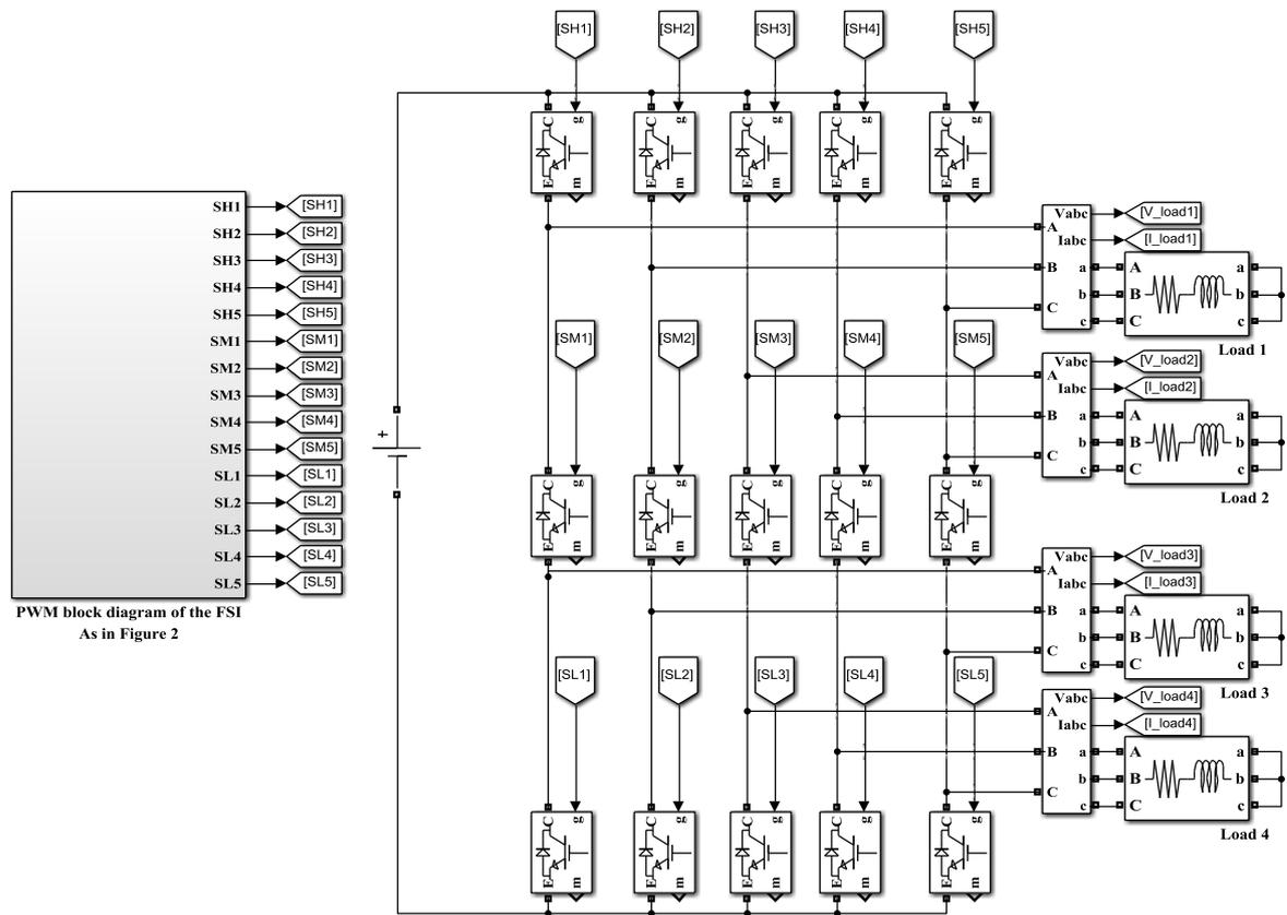
Figure 3. Simulink model of the proposed FSI
