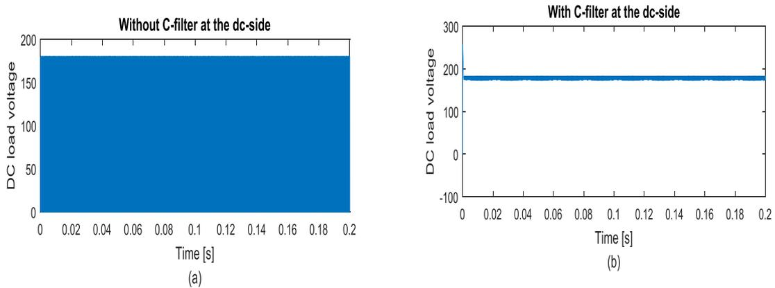
Figure 8. The voltage at the dc-side, (a) without C-filter, (b) with C-filter
