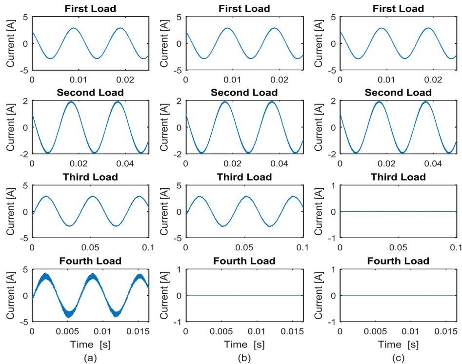
Figure 4. Current waveforms for the four loads, (a) operation mode '1111', (b) operation mode '1110', (c) operation mode '1100'
