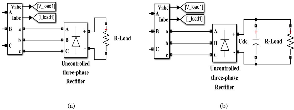
Figure 7. Simulink nonlinear dynamic model of load 1, (a) without C-filter at the dc-side, (b) with C-filter at the dc-side
