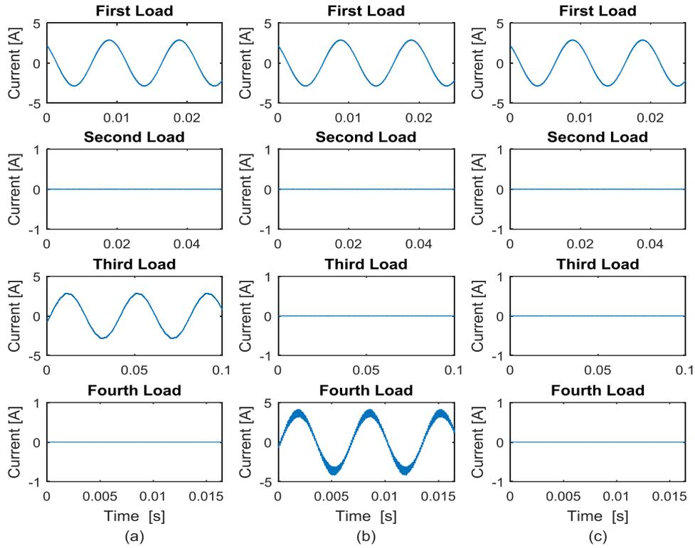
Figure 5. Current waveforms for the four loads, (a) operation mode ‘1010’, (b) operation mode ‘1001’, (c) operation mode ‘1000’
