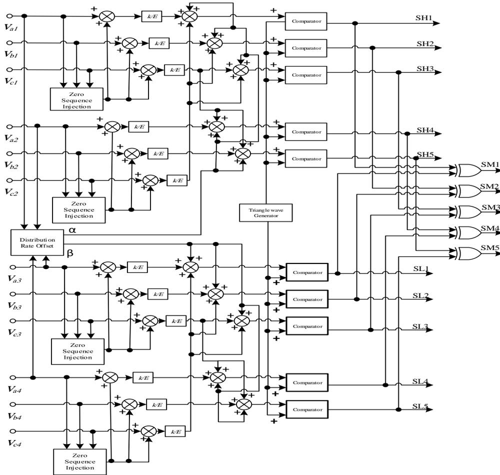
Figure 2. PWM block diagram of the FSI
