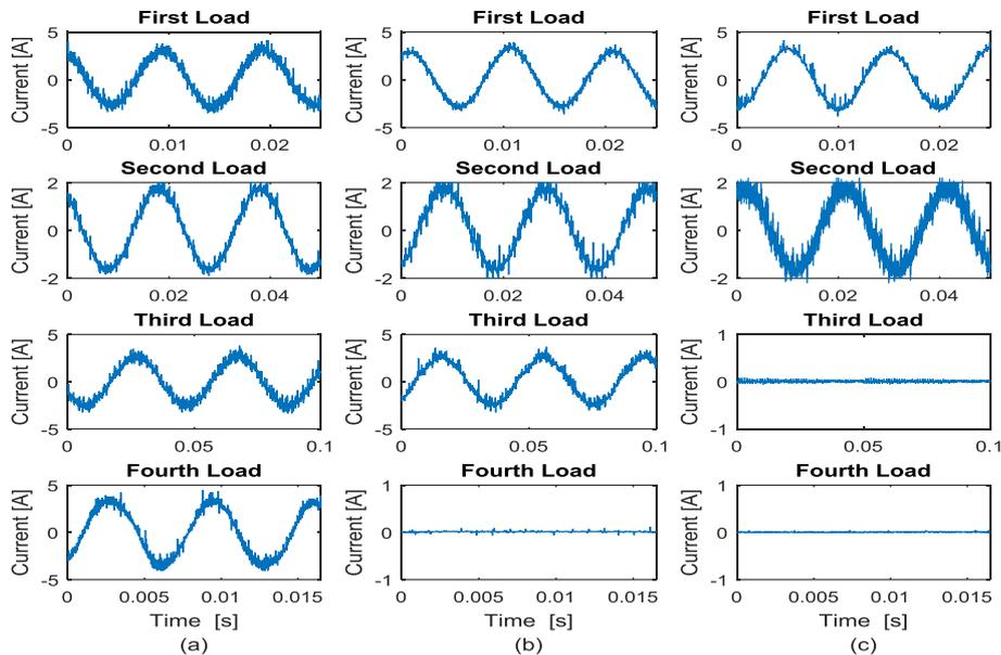
Figure 11. Experimental current waveforms for the four loads (a) Operation mode '1111', (b) Operation mode '1110' (c) Operation mode '1100'
