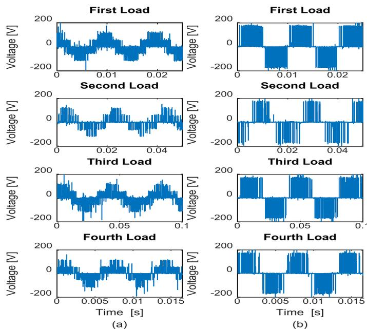
Figure 13. Experimental voltage waveforms for operation mode ‘1111’, (a) phase voltages, (b) line voltages
