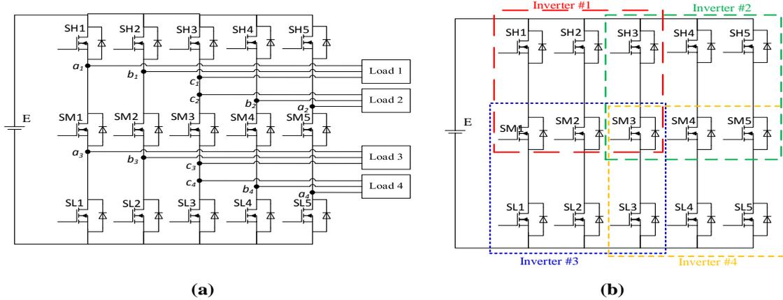
Figure 1. The proposed fifteen-switch inverter, (a) the schematic diagram, (b) the inverters encapsulated in the FSI
