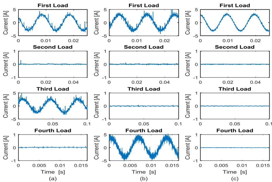
Figure 12. Experimental current waveforms for the four loads, (a) operation mode ‘1010’, (b) operation mode ‘1001’, (c) operation mode ‘1000’
