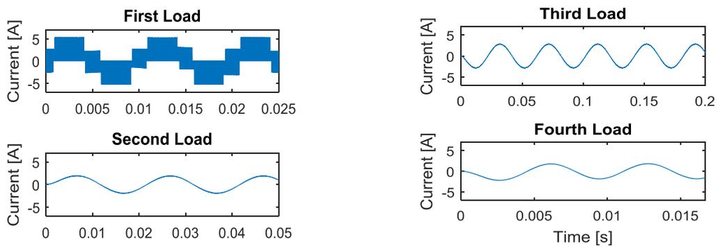
Figure 9. The phase currents of the four loads without adding C-filter at the dc-side
