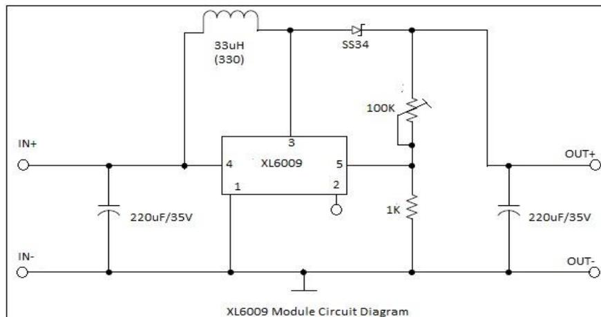
Figure 3. Boost up converter circuit
