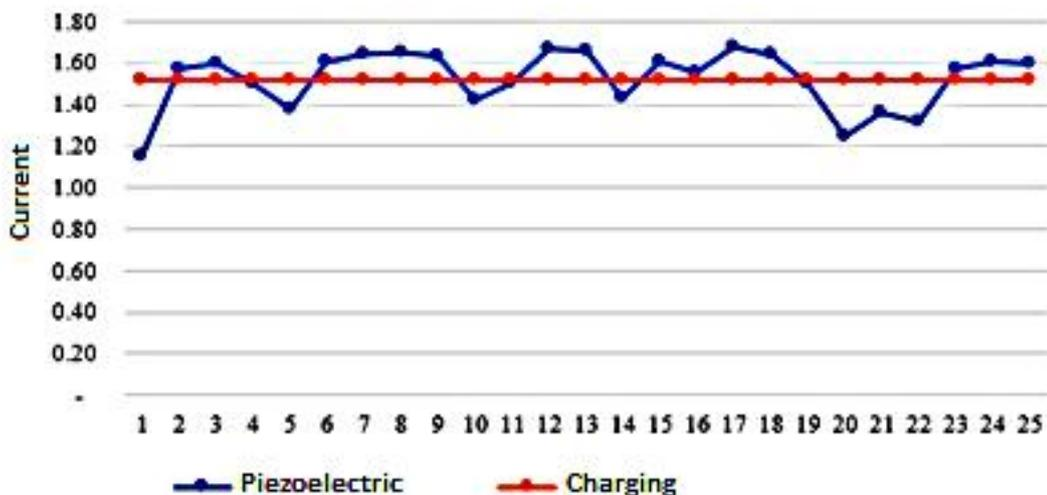
Figure 8. AA battery test using 40 piezoelectrics in parallel
