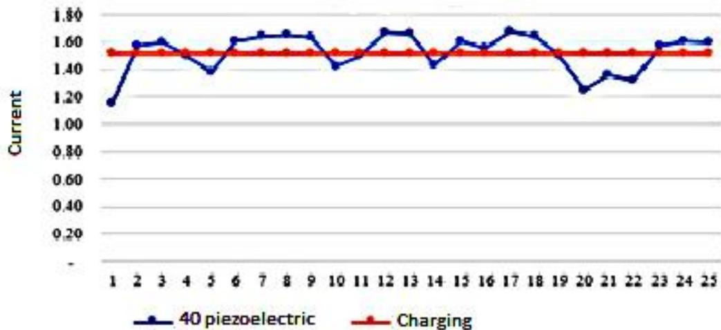
Figure 7. AA battery test using 40 piezoelectrics in parallel
