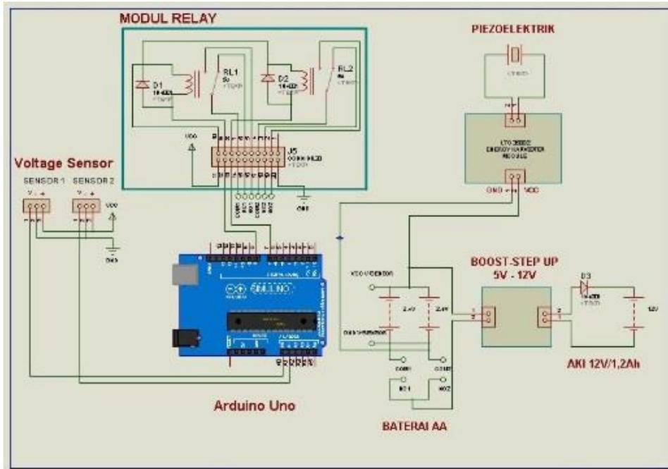
Figure 1. Design of pizeoelectric energy harvester to charge 12 Volt battery
