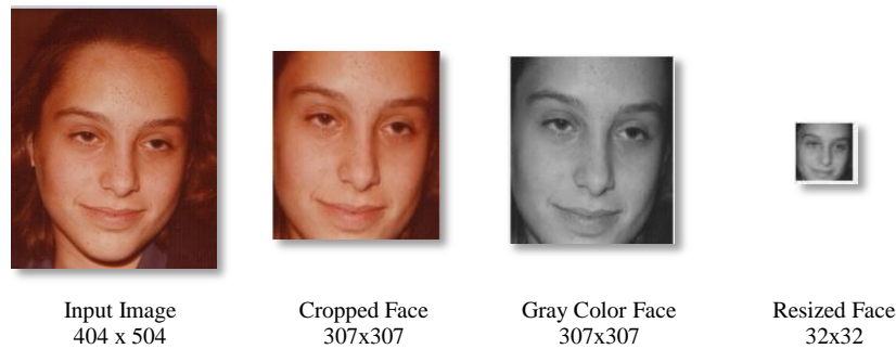
Figure 2. Stepwise Preprocessing for a Sample Image from FGNET Dataset
