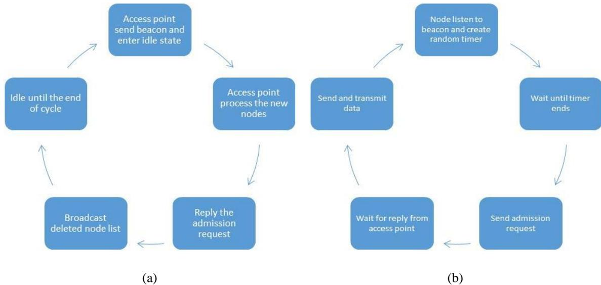
Figure 2. (a) Process flow of access point, (b) Process flow of node
