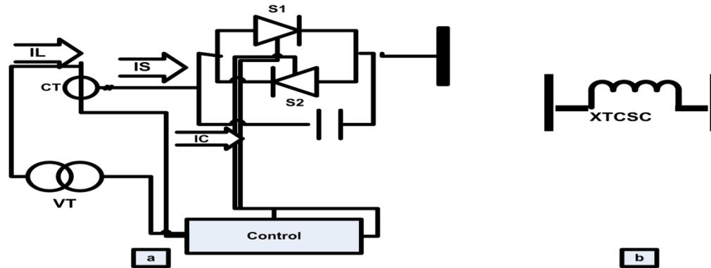
Figure 1. TCSC model connected to Transmission line (a) mounting and (b) apparent reactance [10]
