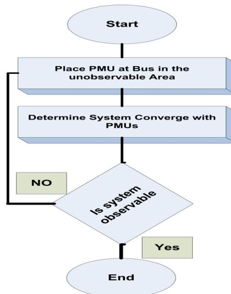
Figure 3. Flowchart of the Graph Theoretic procedure algorithm [18]
