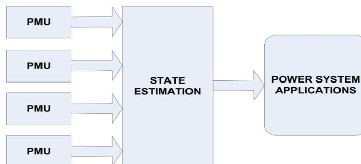
Figure 2. General diagram for state estimation in powersystem operation [13]
