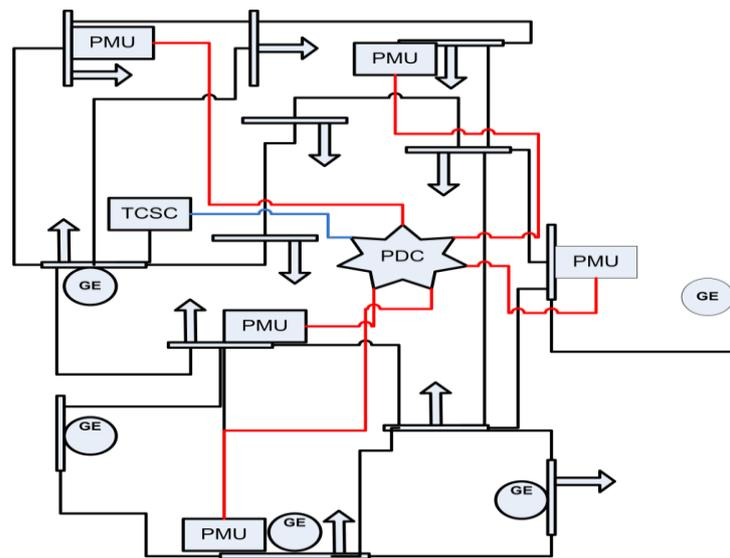
Figure 4. TCSC control with PMU Application on PS. Network
