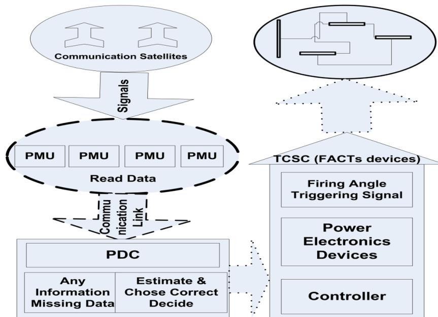
Figure 5. Basic scheme for PMU with FACT’s control (Proposed method)
