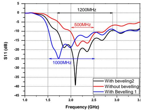
Figure 11. Bandwidth improvement by using beveling technique
