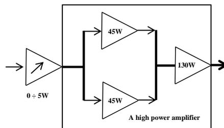
Figure 3. The structure of the Power Amplifier
