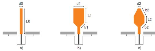
Figure 10. Feed probes of the horn antenna
