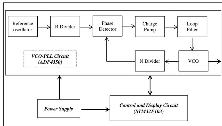
Figure 4. The block diagram of the frequency synthesizer
