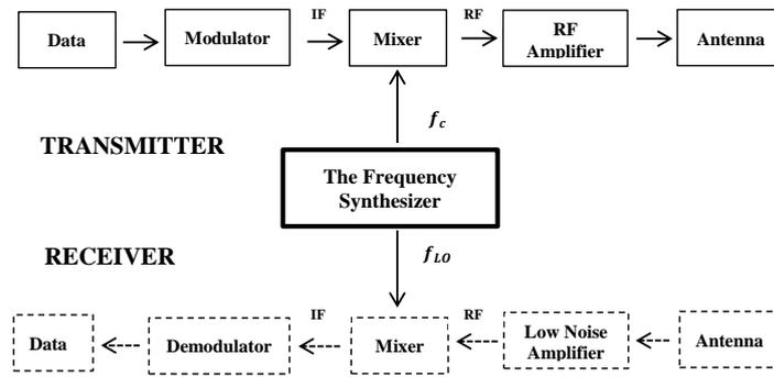
Figure 1. The proposed status data transmitting system
