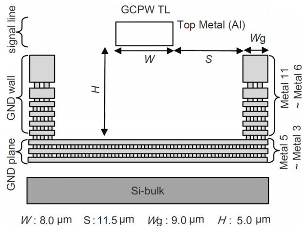
Figure 3. The cross-view of the 50  $\Omega$  GCPW-TL.
