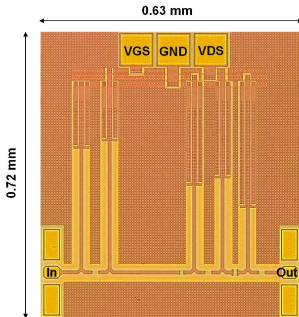
Figure 5. The die microphotograph of the 60 GHz PA.
