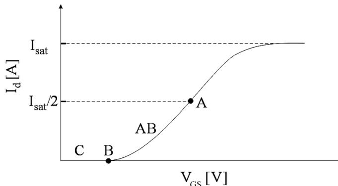
Figure 2. Operating points of different current-mode PAs classes.
