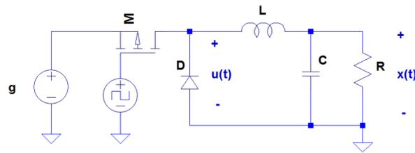
Figure 2. Buck converter circuit
