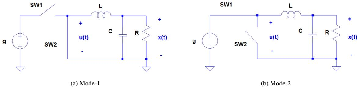
Figure 3. Modes of Buck converter
