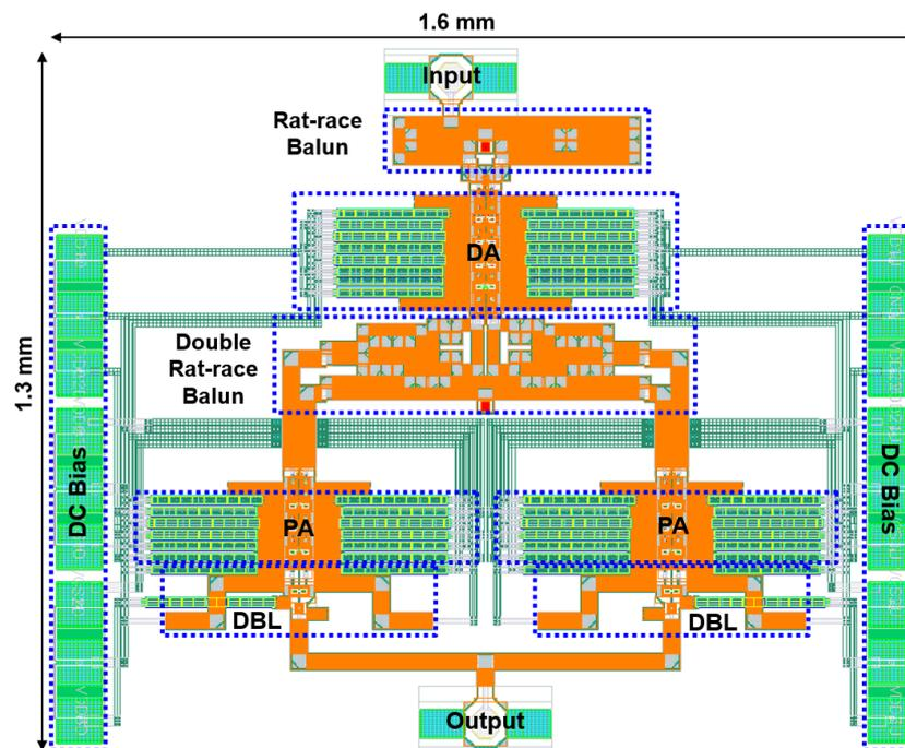
Figure 14. The layout of the 300 GHz transmitter front-end.
