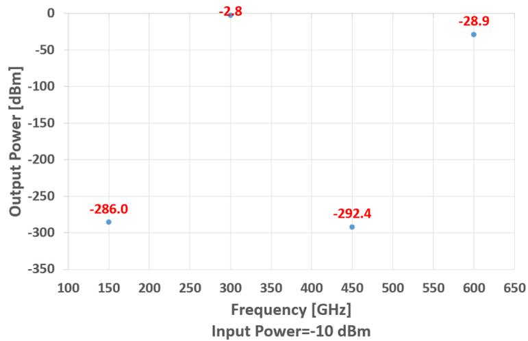
Figure 13. The simulated harmonics of the 300 GHz transmitter front-end.
