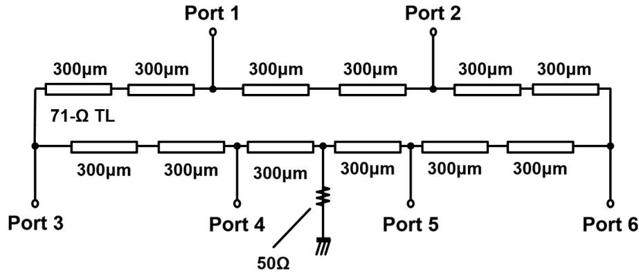
Figure 3. The 150 GHz double rat-race balun.
