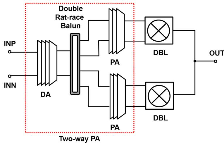
Figure 1. The proposed 300 GHz transmitter front-end.
