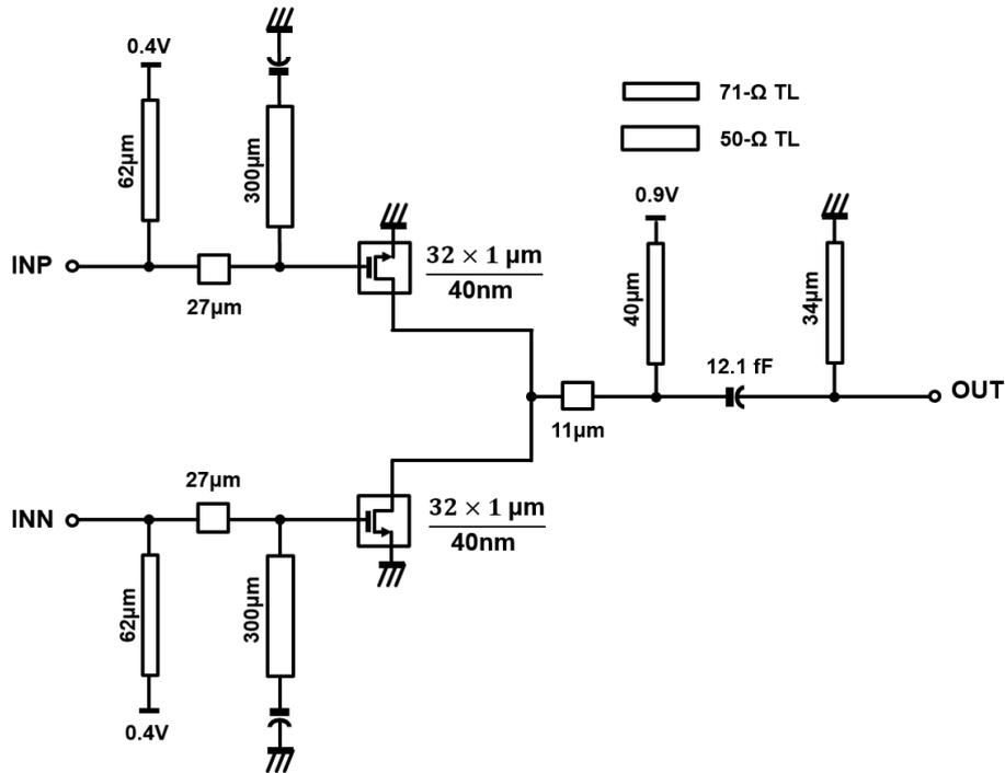
Figure 6. The proposed 300 GHz CS based doubler.
