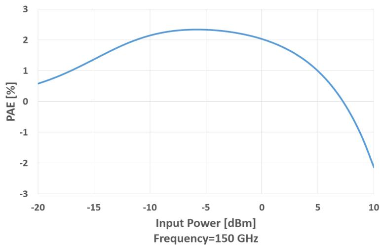
Figure 9. The simulated PAE versus input power of the two-way D-band PA.
