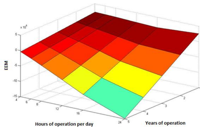
Figure 5. EEM of 100 hp for 1-5 years “-ve” new motor and “+ve” rewind motor is the best replacement
