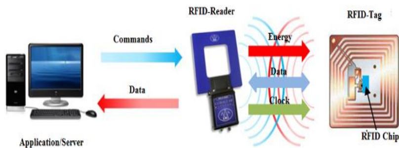
Figure 1. Block Diagram of an RFID System
