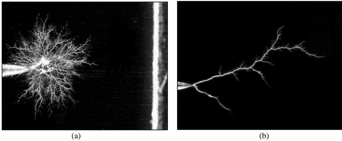
Figure 1. Treeing Structures, (a) at 20% relative humidity and (b) at 90% relative humidity
