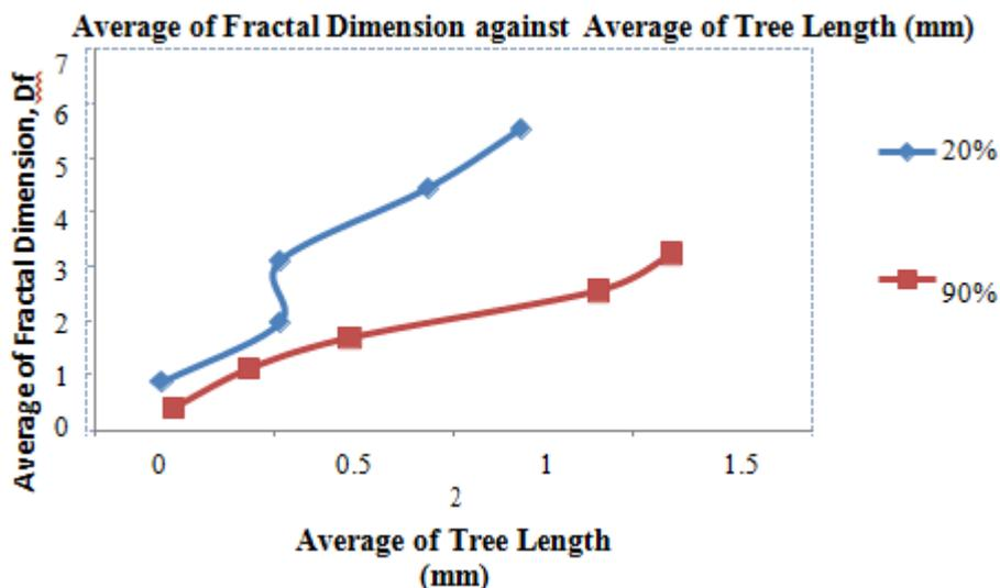
Figure 3. Tendency of fractal dimension to the function of tree length at 20% and 90% relative humidity
