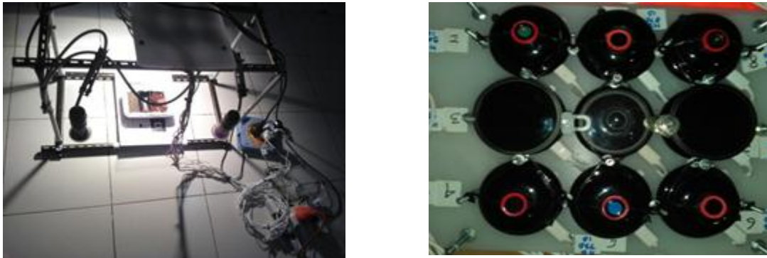
Figure 2. On the left is the instrumentation setting and on the right is nine cameras and its associated optical filters
