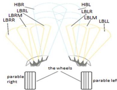
Figure 4. lighting trajectories for different lamps
