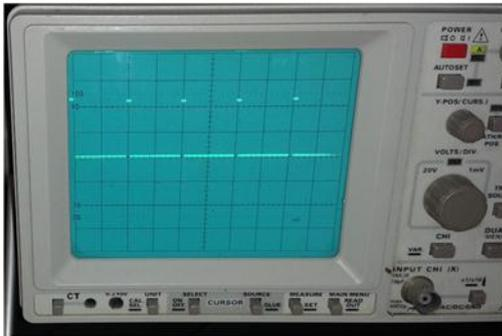
Figure 10. Example of a signal PWM duty cycle of 7.8% generate by ARDUINO
