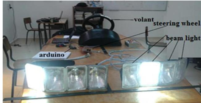
Figure 11. Prototype realized of AFS system
