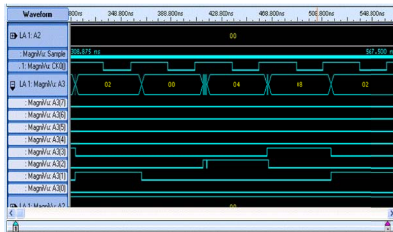
Figure 4. Output Signal of Integrated System (Addition Process) for N = 4 and WI = 4
