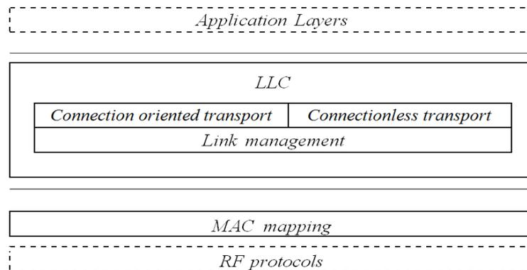
Figure 1. OSI models for NFC peer-to-peer mode [5]
