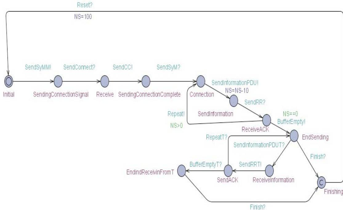
Figure 3. Communication of LLCP layer with TA method
