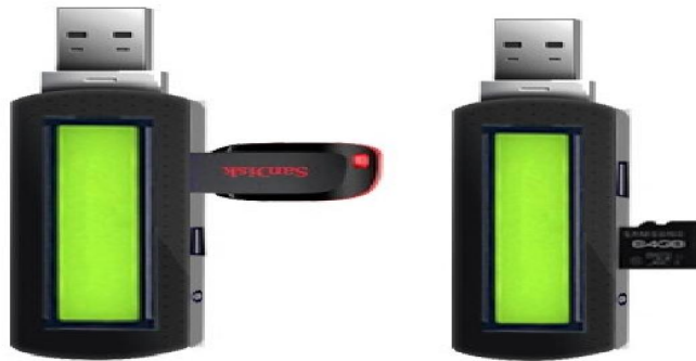
Figure 12. Data Transmission through USB &SD card slot
