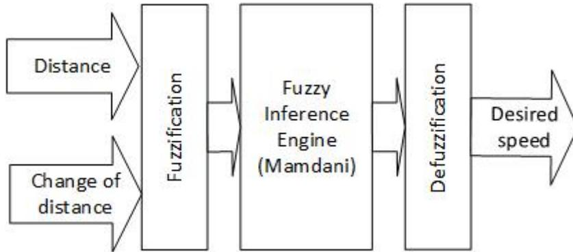
Figure 4. Block diagram of a high-level controller based on fuzzy logic
