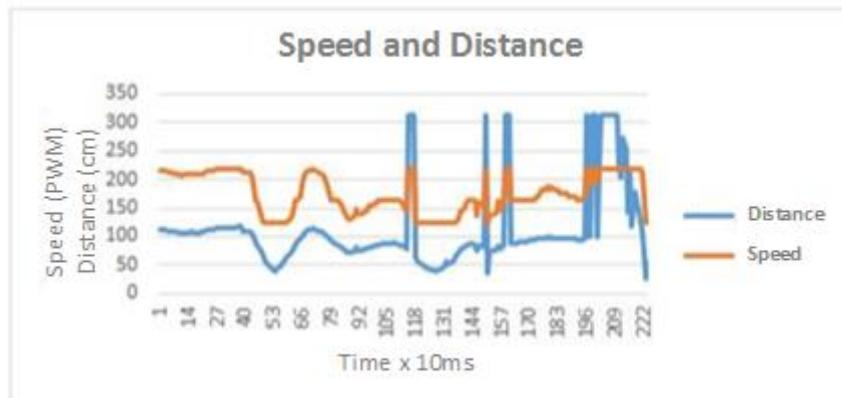
Figure 16. ACCtest data with speed of LV changeable
