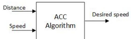
Figure 3. High-level controller of the ACC using double inputs
