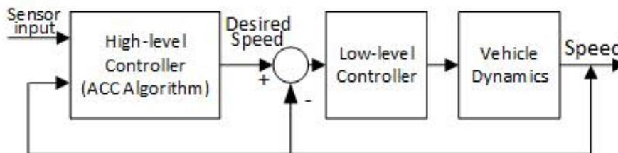
Figure 1. Block diagram of the ACC
