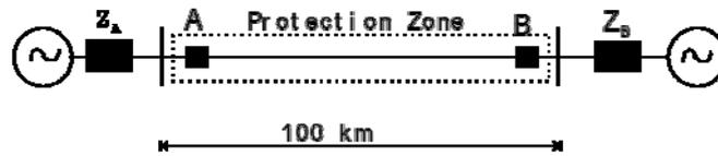
Figure 1. Transmission line model
