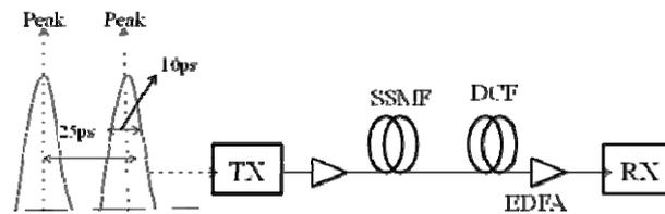
Figure 1. Transmission line models for a DM system
