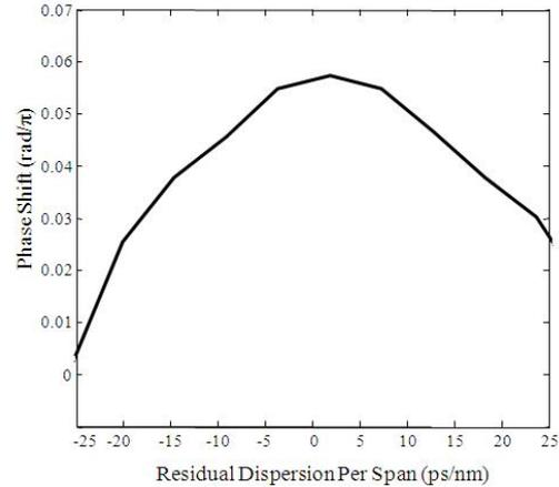
Figure 7. Phase shift versus residual dispersion per span for dispersion managed system
