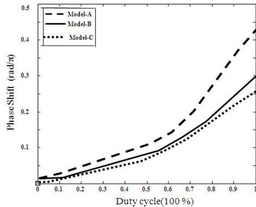
Figure 5. Effect of duty cycle on IXPM induced phase fluctuation for three models
