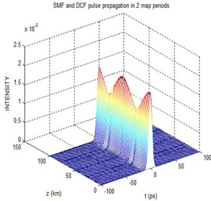
Figure 2. Single Pulse dynamics within the DM system with full numerical simulation
