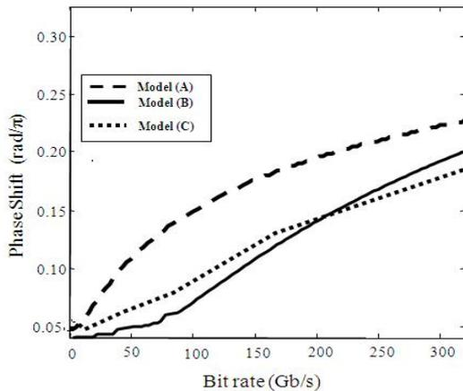
Figure 6. IXPM induced Phase fluctuation as a function of bit rate for three models
