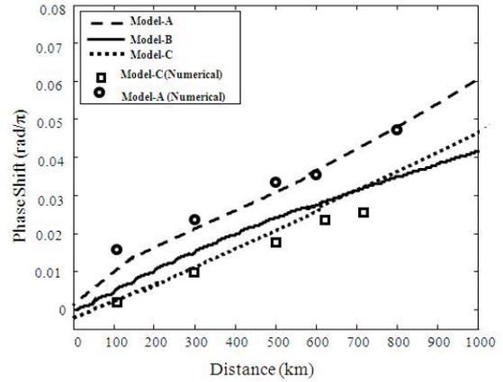
Figure 3. Phase fluctuation against transmission distance for different residual dispersion.
