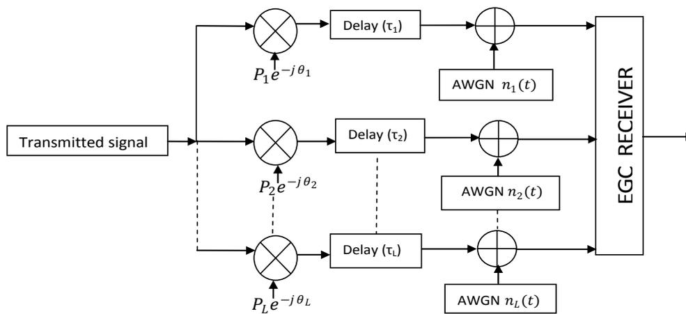
Figure 1. Multilink Satellite Flat-Fading channel model
