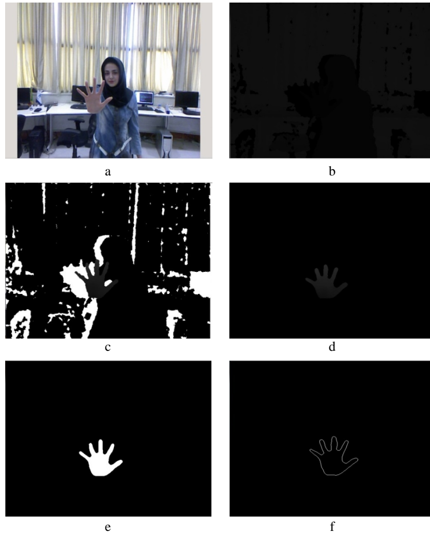
Figure 2. (a) Original color Image in clutter background (b) Depth Image. (c) Rescaling Image (d) Median Filtering (e) Thresholding (f) Hand contour
