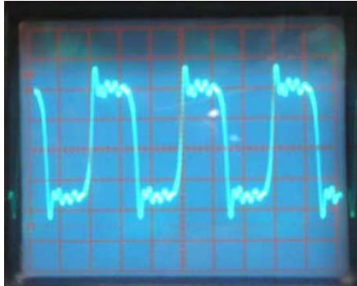
Figure 13. Input of the bridge rectifier
