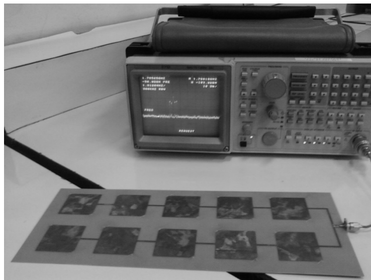
Figure 5. Measurement of Circularly-Polarized Microstrip Array Antenna at 1800 MHz
