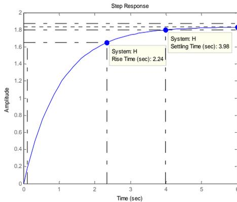
Fig.6. Step response of PMH motor for Topology 6
