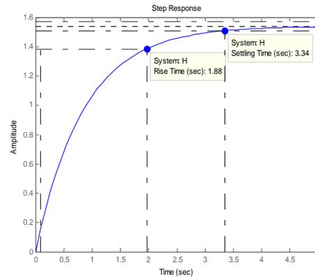
Fig.7. Step response of PMH motor for Topology 8
