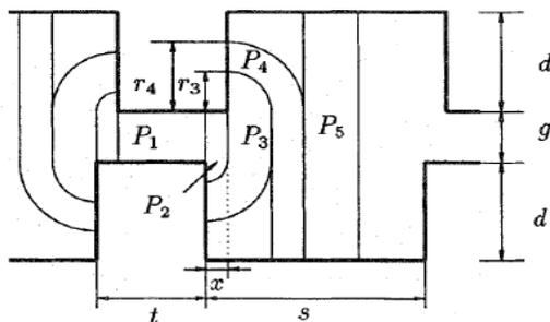
Fig.1.Linearized tooth layer unit arrangement and flux tubes
