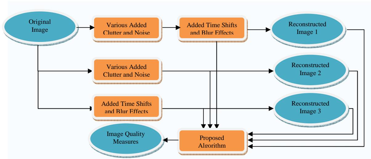
Figure 3. The validation approach functional block diagram for the proposed algorithm for blind image quality assessment
