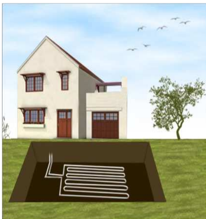
Figure 6. Closed Pond (lake) loops system
