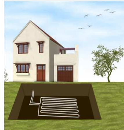
Figure 5. Closed Horizontal loop system
