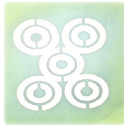
Figure 14 (a). Fabricated “SPLIT RING” shaped metamaterial structure at a height of 3.2mm from the ground plane
