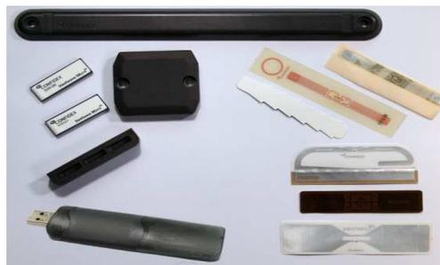
Figure 6. CoreRFID demo kit
