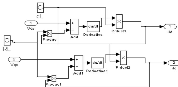
Figure 3. Internal model of balanced capacitive load
