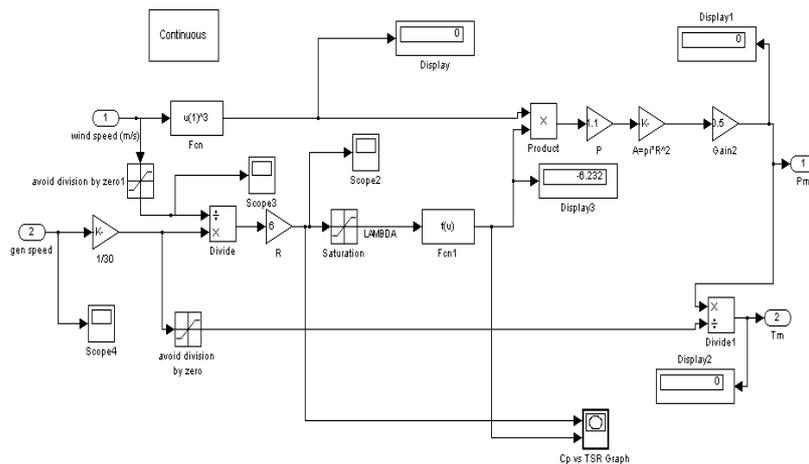
Figure 6. Custom wind turbine model (Air Density: 1.1 kpa)
