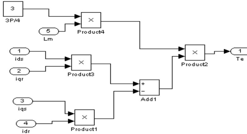
Figure 5. Electromagnetic torque
