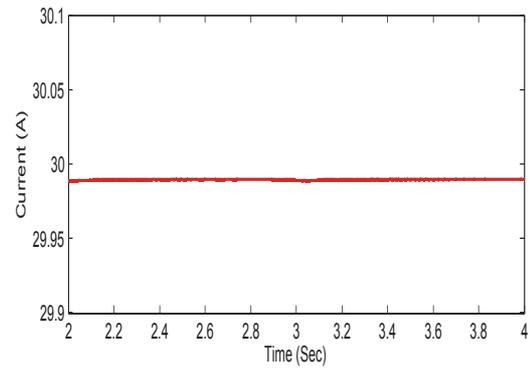
Figure 12. PV cell performance with constant load under constant radiation and temperature (y-axis PV array current (A) and x-axis time)
