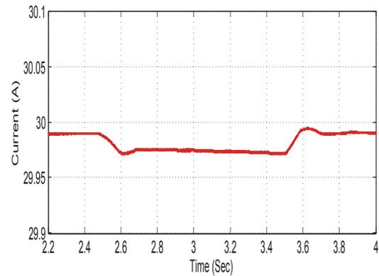
Figure 16. PV cell performance with constant load under variable radiation and temperature(y-axis PV array current (A) and x-axis time)
