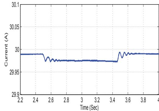
Figure 14. PV cell performance with PHEVs load under variable radiation and temperature (y-axis PV array current (A) and x-axis time)
