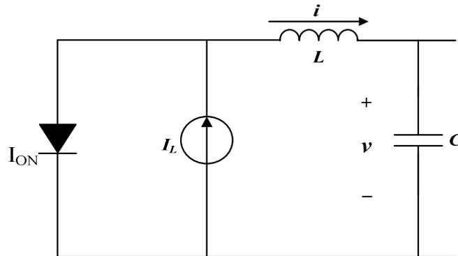
Figure 4. PV equivalent circuit [22]
