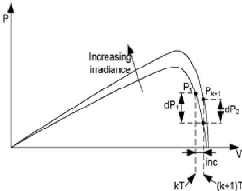
Figure 7. P-V characteristic curve of PV cell with MMP T [26]
