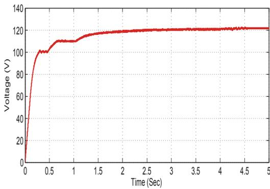
Figure 11. PV cell performance with constant load under constant radiation and temperature (y-axis PV array voltage (V) and x-axis time)
