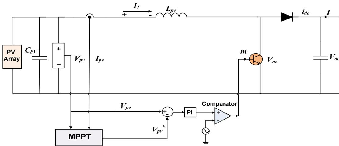
Figure 6. PV converter controller System
