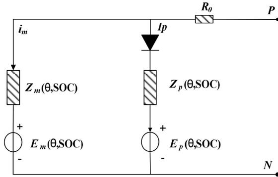
Figure 2. Battery equivalent network with parasitic branch
