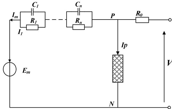
Figure 3. Battery equivalent network
