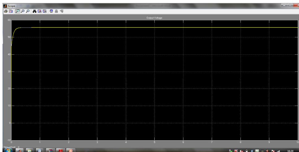
Figure .6 Output Voltage waveform of Boost Converter
