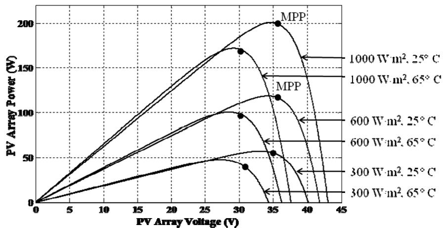
Figure 10. P-V characteristics under different insulations and temperatures
