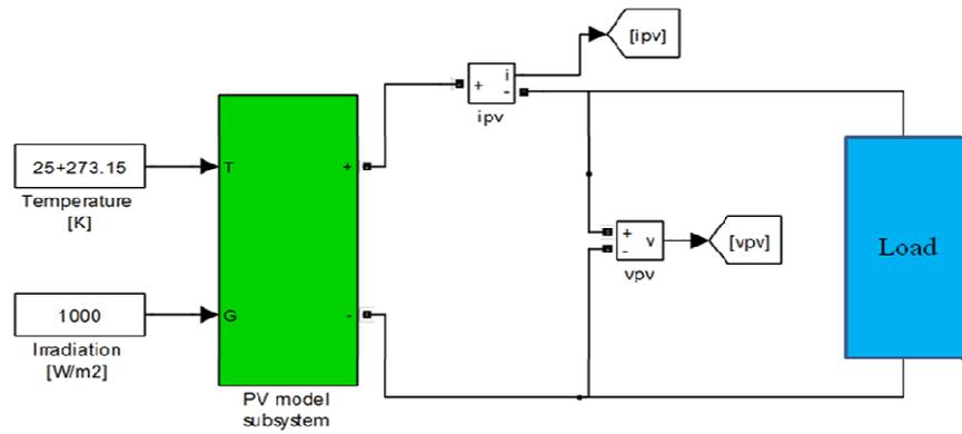
Figure 6. Simulink model of PV array
