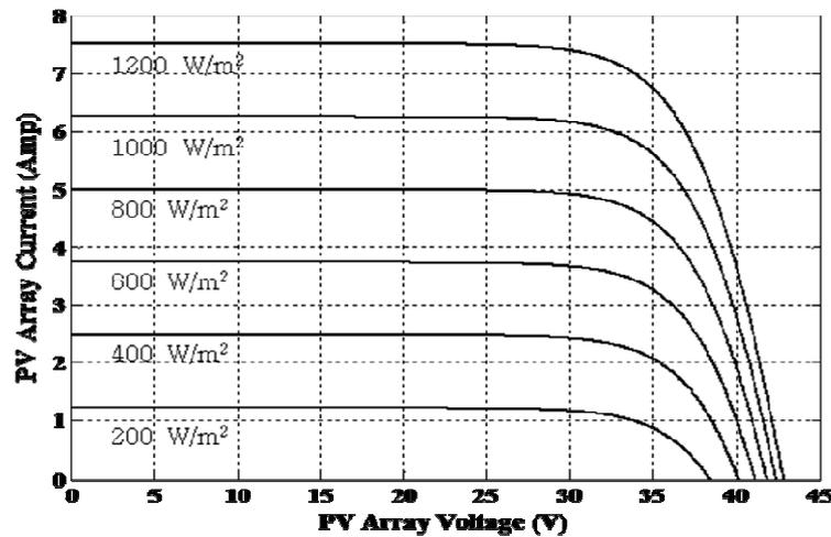
Figure 7. I-V characteristics of the solar PV array due to change in insolation at 25°C
