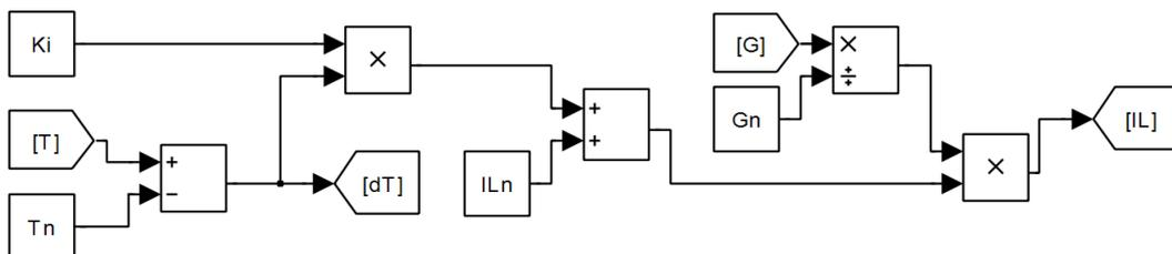
Figure 5. Masked subsystem of light generated current for a single cell
