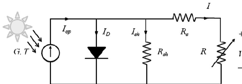
Figure 3. Equivalent circuit of a solar cell consisting of discrete electrical components.
