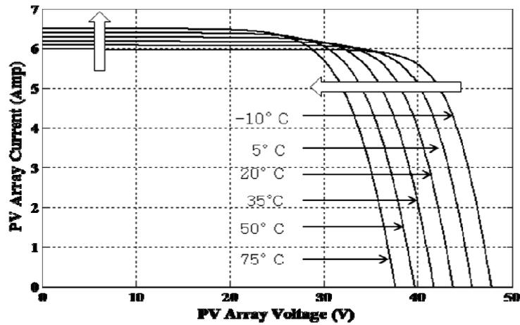
Figure 9. I-V characteristics under different temperatures at solar irradiation of 1000W/m<sup>2</sup>
