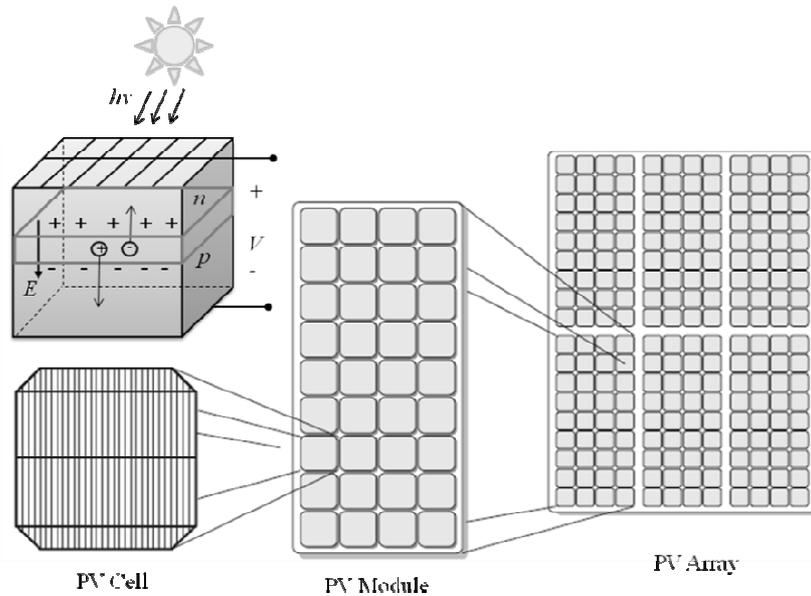
Figure 2. A typical structure of solar PV cell, module and array.
