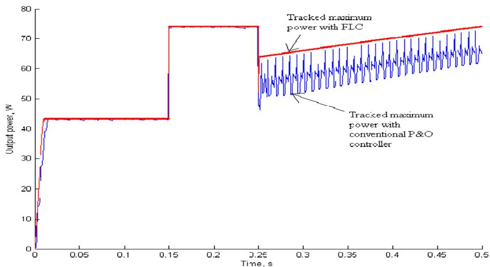
Figure 18. Output power with FLC and conventional P&O controller
