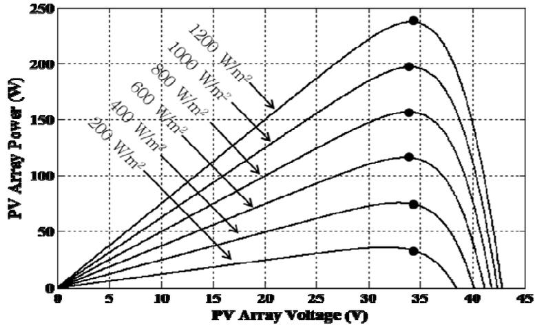
Figure 8. P-V Characteristics of the two series connected PV array due to change in insolation at 25°C
