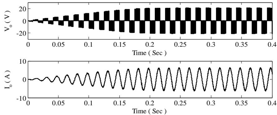
Figure 11. AC Output voltage and current waveforms of the inverter
