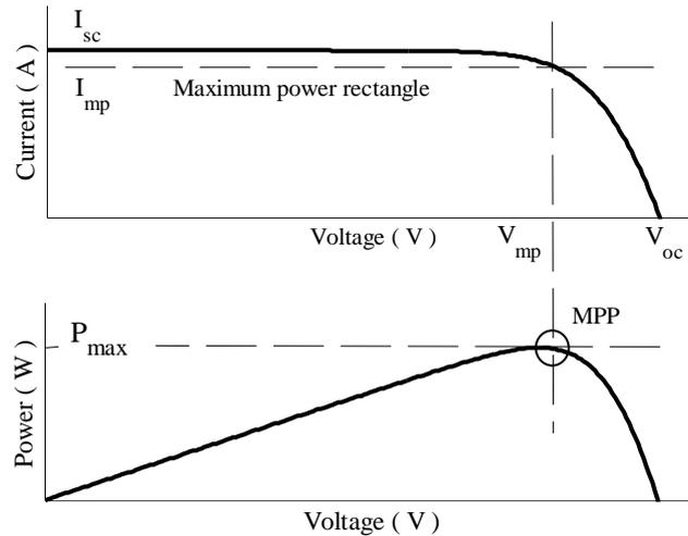
Figure 4. Typical I-V and P-V characteristic and location of  $V_{oc}$ ,  $I_{sc}$ ,  $I_{mp}$ ,  $V_{mp}$ ,  $P_{max}$  and MPP
