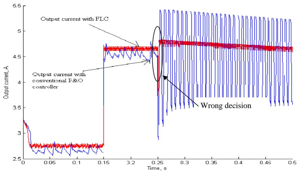
Figure 17. Output current with FLC and conventional P&O controller
