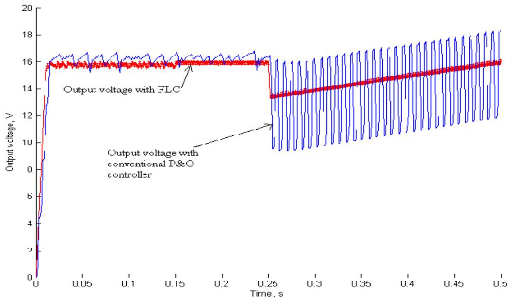
Figure 16. Output voltage with FLC and conventional P&O controller
