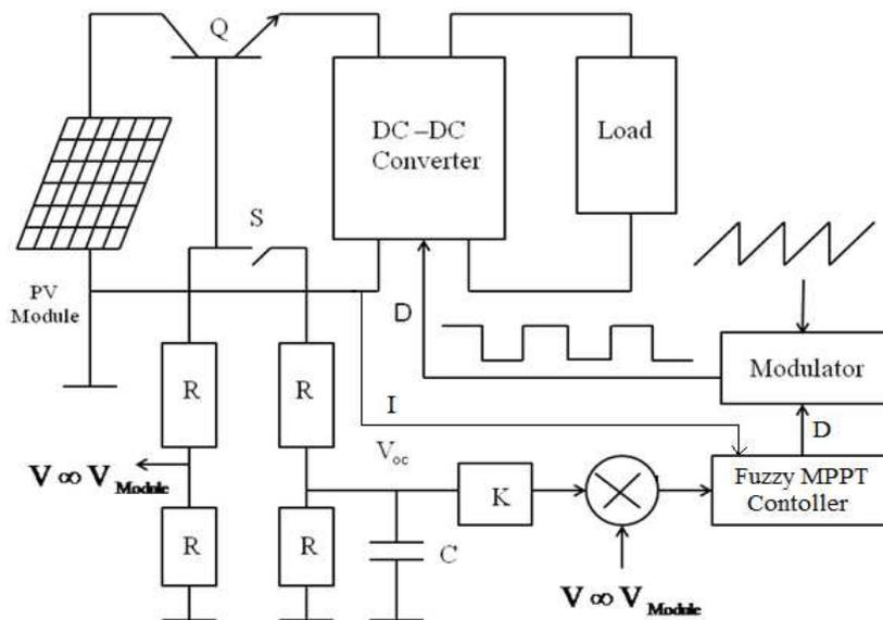
Figure 12. PV array with General MPPT system
