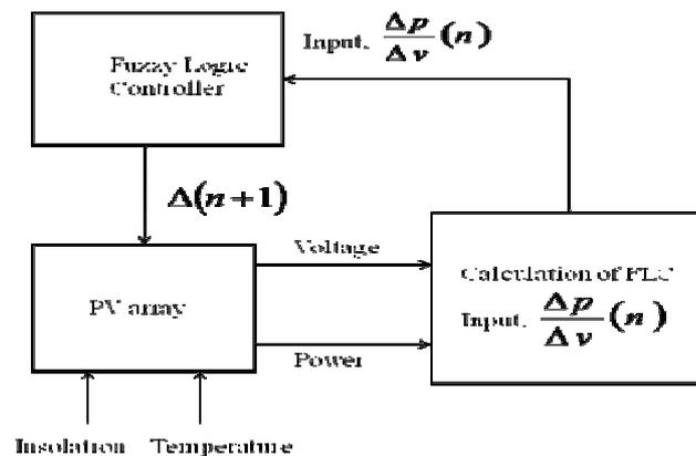
Figure 13. Functional block of FLC based MPPT system [20]
