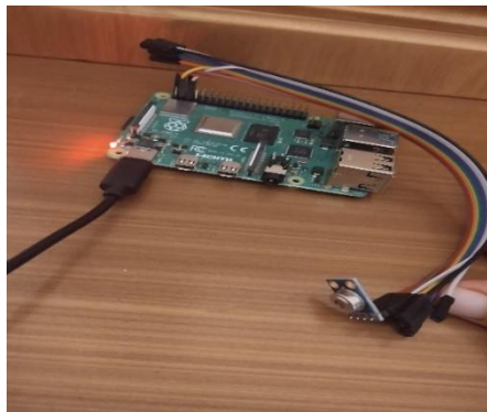
Figure 3. Connecting IoT components: Raspberry Pi 4 board, Dupont cable, MLX90614 sensor
