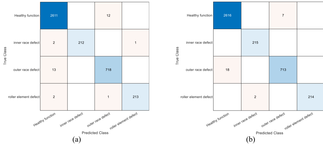
Figure 3. The confusion matrix for the best performers, (a) random forest and (b) ANN
