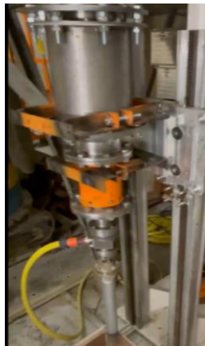
Figure 1. Prototype of rotary drilling rig
