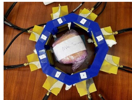
Figure 8. Image of the experimental setup, including the Vivaldi antennas and the breast-mimicking phantom
