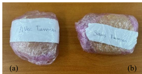
Figure 2. Realistic breast models for microwave imaging (developed in our laboratory) (a) breast with tumor and (b) healthy breast
