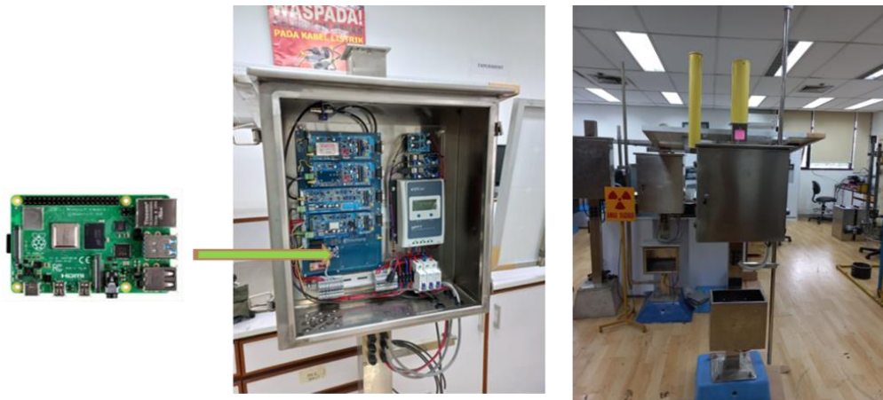
Figure 7. Raspberry pi hardware integrated into environmental monitoring station
