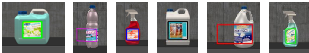
Figure 5. Results of SURF algorithm applied to different products formats with their respective labels
