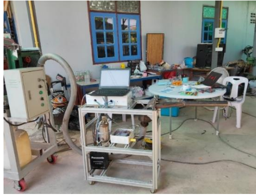
Figure 6. Experimental setup for gas production monitoring
