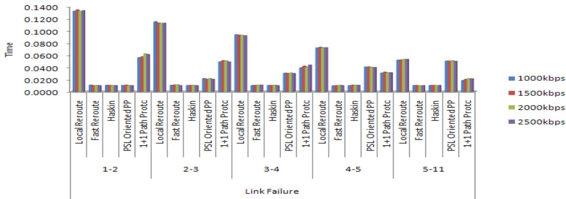
Figure 11 Comparison of recovery time from the five mechanisms
