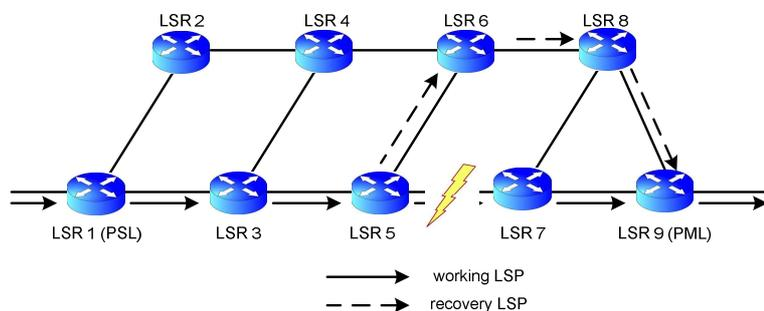
Figure 3. Local Rerouting Mechanisme [17]
