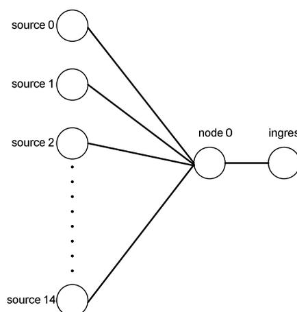
Figure 1. Aggregate Traffic Generation Topology
