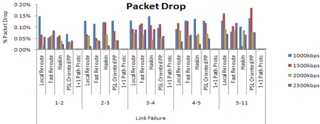
Figure 8. Comparison of packet drop at the five mechanisms
