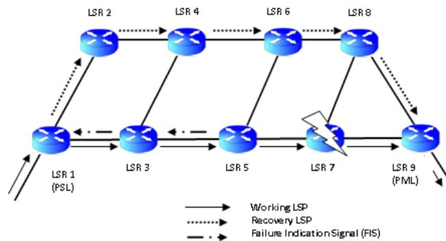
Figure 6. PSL-Oriented Path Protection Mechanism
