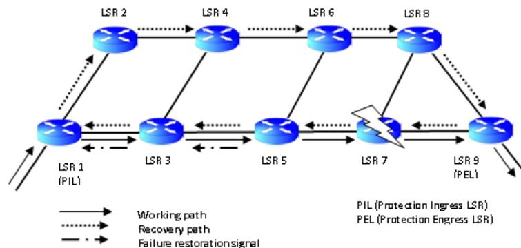
Figure 5. Haskin Recovery Mechanism [17]
