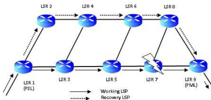
Figure 7. Recovery 1+1 Path protection Mechanism [1]
