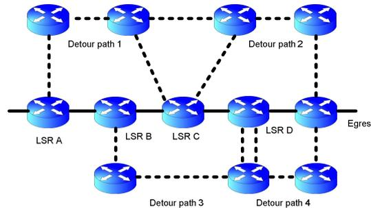
Figure 4. Detour Fasterroute One-to-One Backup [5]
