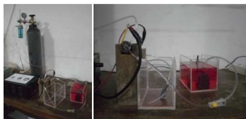
Figure 9. Test of Ozone reactor with wire-cylinder electrode configuration.
