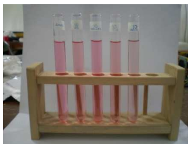
Figure 17. Comparison result of the tenth cycle of wastewater treatment process in each high-voltage Ozone reactor (left to the right): (a) initial wastewater before the treatment process; (b) Ozone reactor with wire-cylinder configuration; (c) Ozone reactor with spiral-cylinder configuration; (d) Ozone reactor with DBD wire-cylinder configuration; (e) Ozone reactor with DBD spiral-cylinder configuration
