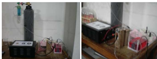
Figure11. Test of Ozone reactor with spiral-cylinder electrode configuration
