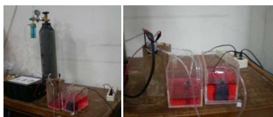
Figure13. Test of Ozone reactor with DBD wire-cylinder electrode configuration
