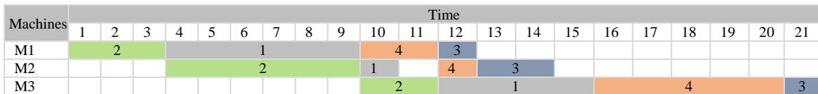
Figure 3. Gantt chart of initial solution 2-1-4-3 (S= (2-1-4-3))
