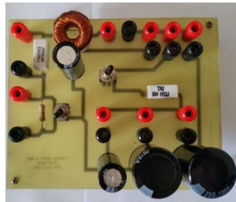
Figure 5. DC system model with RC parallel passive damping Figure 6. Hardware circuit implementation
