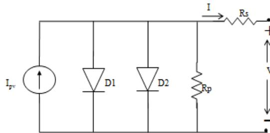
Figure 1. Two diode model of the PV Cel
