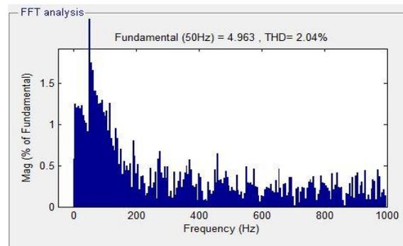
Figure 27. THD Analysis of the Grid Current
