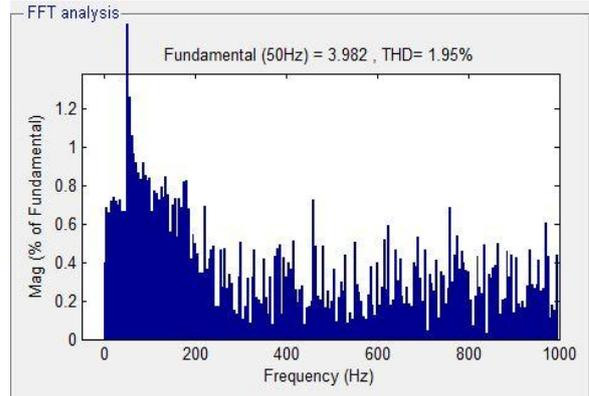
Figure 19. THD analysis of the Grid Current
