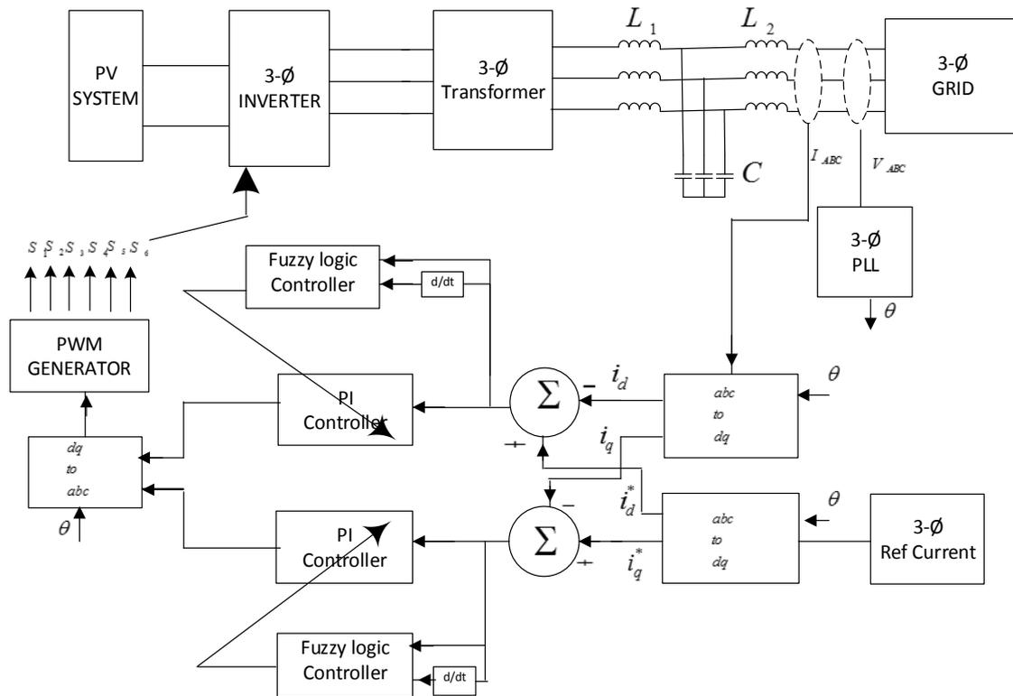
Figure 3. Overall Block Diagram of the PV Inverter Connected to the grid with Adaptive Fuzzy PI Controller
