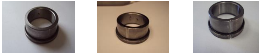
Figure 7. Failure on the inner ring of the bearing NUP 206 (a-Level 1/3, b- Level 2/3 and c- Level 3/3)
