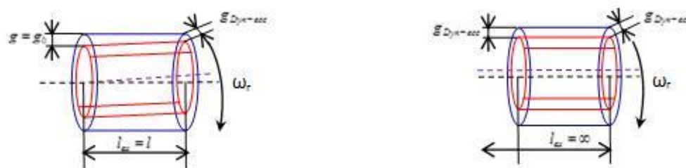
Figure 1. Non uniform (left) and uniform (right) dynamic air gap eccentricity
