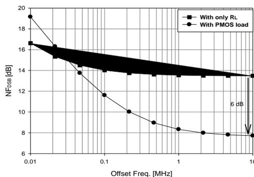
Figure 5. Simulated double sideband (DSB) noise figure of the single balanced mixer with and without the PMOS load
