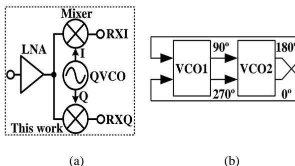
Figure 1. (a) Receiver RF front-end and (b) quadrature signal generation with two differential VCOs
