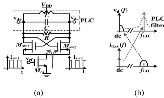
Figure 2. (a) Conventional PLC VCO as a mixer and (b) its frequency response
