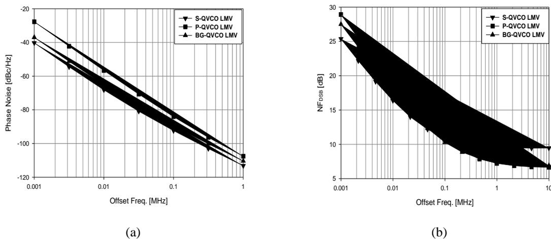
Figure 10. (a) Phase noise and (b) double sideband noise figure of the proposed QVCO LMVs
