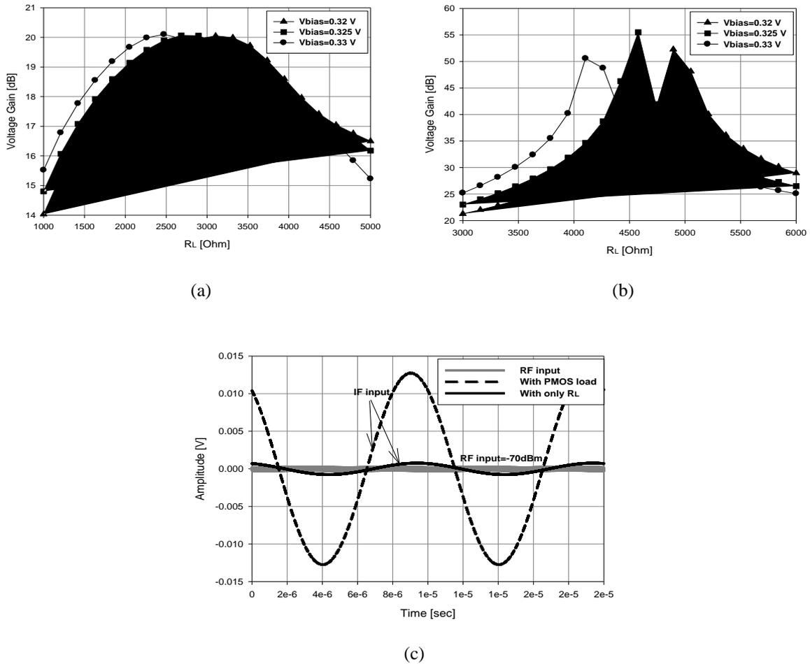
Figure 4. Simulated voltage gain (a) load resistor only, (b) load resistor added with PMOS active load, and (c) the signal swing comparison with and without PMOS load
