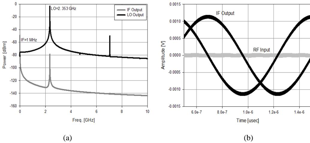
Figure 9. (a) Frequency domain analysis of the S-QVCO LMV, (b) Voltage swing at the RF input and IF output of the S-QVCO LMV. The applied RF input power is  $-80$  dBm
