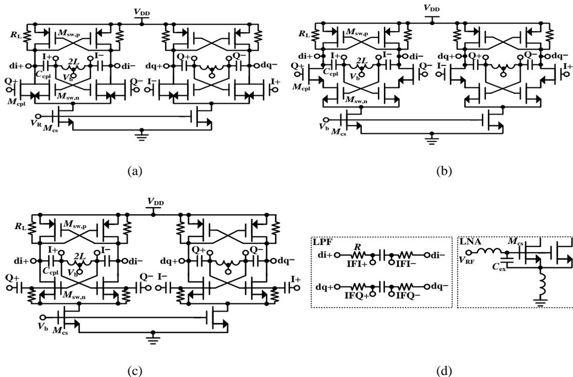
Figure 7. Proposed QLMVs. (a) P-QVCO LMV, (b) S-QVCO LMV, (c) BG-QVCO LMV, and (d) LPF and LNA
