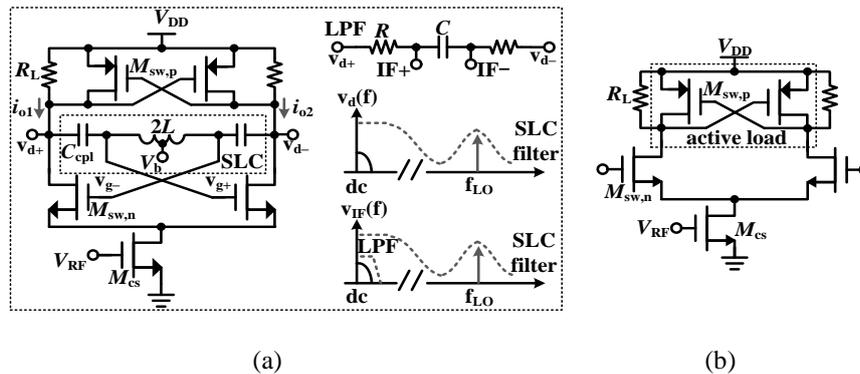
Figure 3. (a) Single-balanced (SB) SLC VCO as a mixer with its frequency response [6] and (b) single-balanced mixer with PMOS active load
