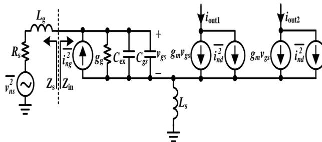
Figure 8. Small-signal equivalent circuit of the LNA
