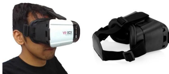
Figure 2. VR Box Virtual Reality Head Mounted Display (HMD) [13].
