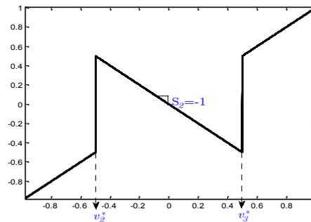
Figure 4. Nonlinear hard element  $f(\cdot)$  considered in simulation.
