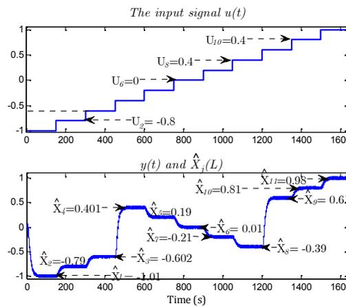
Figure 5.  $u(t)$ ,  $y(t)$  and the undisturbed output estimate.
