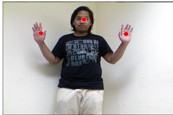
Figure 2. Kinect presentation control with hand tracked
